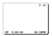
2 To remove the status display, press the **DISPLAY** button (press the button twice if a tape is loaded in the VCR).
